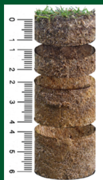
Picture no.2: Soil core sample with incremental depths
